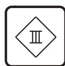
**GB** Protection class 3: the fitting is suitable only for low voltage, e.g. 12V.
